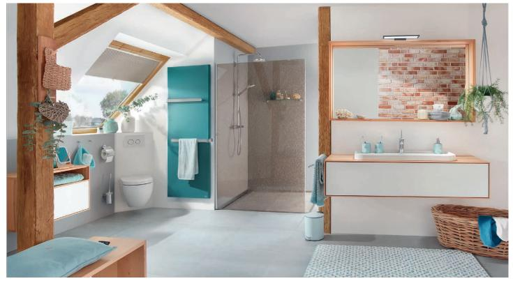
An unused attic becomes an "oasis". The available low heights of the **Grumbach corner WC-block** allow installation on the jamb. The spacious, floor-level shower area is realized with the help of the **120** x **120** cm shower floor element made of PUR with channel drainage and height-adjustable side panels.
