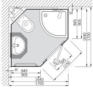
Pre-fabricated bathroom UNIVERSAL is the ideal solution for installation in the corner. It requires less than 3 m<sup>2</sup> floor space!
