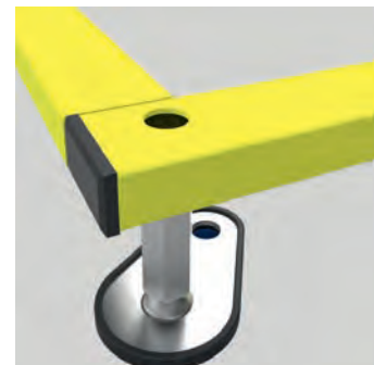
Adjustable feet for simple positioning and fastening: with layer of rubber for the de-coupling of structure-borne noise. The number of adjustable feet depends on the frame size.
