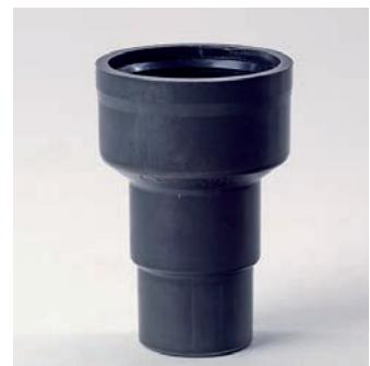
Reducing piece made of PUR, internal rubber seal (like sleeve), suitable for the attica Jumbo drain with adapter for the reduction of the nominal width from DN 150 to DN 125 or 100.
