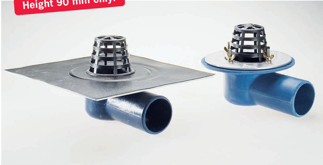
The **Garage/Balcony drains** distinguish themselves through their particularly small and compact appearance with a support diameter of DN 70; this is the case with the clamp flange and the adhesive collar version. The horizontal drain is especially suitable for many problematic situations on balconies, loggias and small roofs, due to its **particularly low construction height**.
