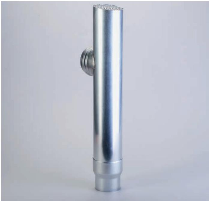
Attica downpipe connection made of titanium zinc DN 70 in combination with a reducer from Ø 87 mm to Ø 80 mm.
