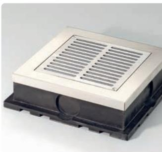
Green roof safety drain made of PUR, 365 x 365 mm, with pre-formed connections for drainpipe Ø 70 mm and sieve panel made of aluminum. Height 100 mm
