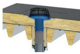
Compact fire protection drain DN 100 with inserted Eco drain top part in the trapezoid sheet roof with insulated roof construction.
