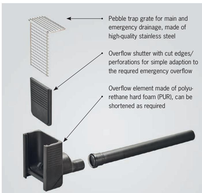
Example: Attica plug-in overflow in the attica balcony drain with partial flow diversion made of stainless steel (for direct downpipe connection)
