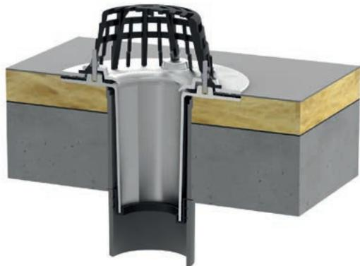
Redevelopment drain made of aluminum DN 90 for the redevelopment of sleeveless pipes and roof drains DN 100 without applying extra insulation.
