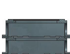
The green roof safety drain small can be stacked as required.
