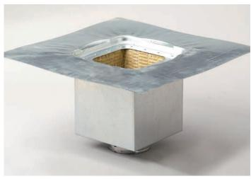
Grumbach fire protection element for roof drains – **optimally adapted for the universal and compact collar drain series** from Grumbach. The fire protection cladding is shaped with a quadruple impression/recess on top, thus allowing an optimal positioning of the drain, water can then drain completely, without backing-up at the drain flange.
