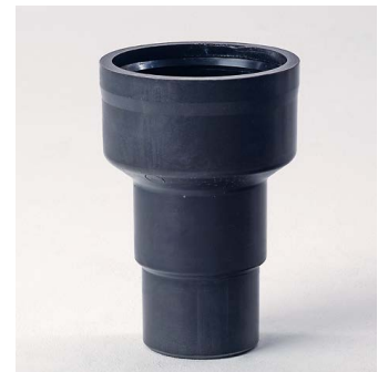
Reducing piece made of PUR, internal rubber seal (like sleeve), suitable for the attica Jumbo drain with adaptor for the reduction of the nominal width from DN 150 to DN 125 or 100.
