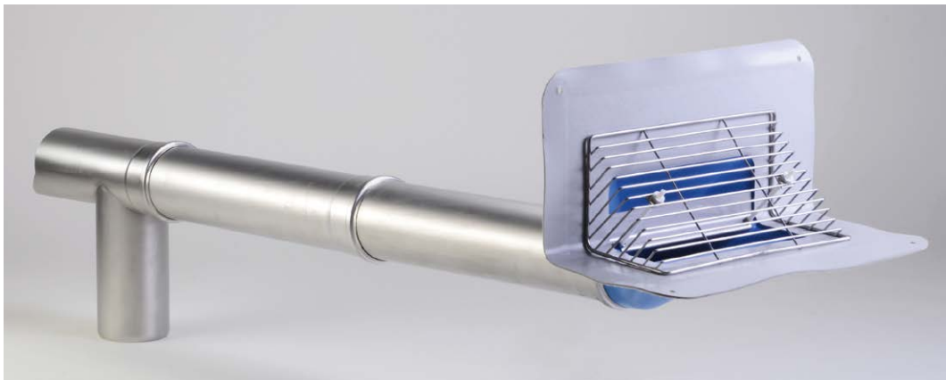
Attica Super-2 drain without wedge with partial flow diversion (long version). The version without a wedge is available with various connection collars.
