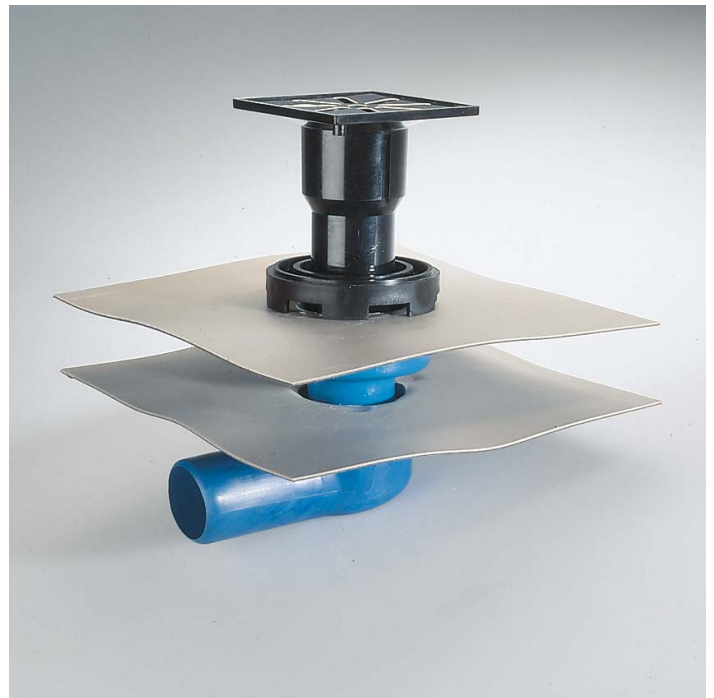
Balcony drain, horizontal DN 50, with extension element with adhesive collar , pebble trap and inlet piece, which is able to be walked upon. For use on balconies, for example.
