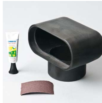
Adaptor for attica Jumbo drain made of PUR with connection supports for a sleeve pipe DN 150. For on-site connection to an attica Jumbo drain. Sandpaper and adhesive are included in the scope of delivery.
