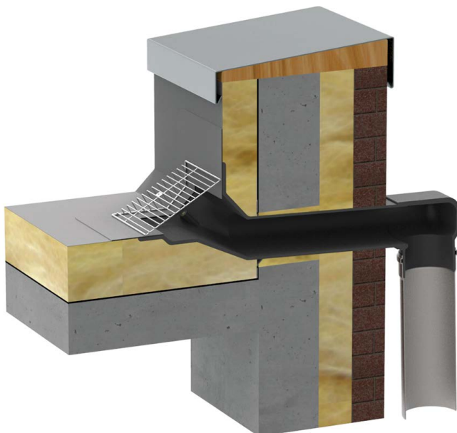
Attica Jumbo drain with adaptor and connecting piece for vapour traps fastening cuff in the insulated roof. To prevent frost damage, we recommend using our trace heating systems (see page 74).
