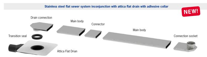
With the new **transition seal** (shown in red), the flat sewer system can be connected to the attica flat drain with adhesive collar. The **transition seal made of EPDM** tapers the cup area of the drain to DN 100 so that the drain connection of the flat sewer system (or bends, pipes or standpipes) can be inserted tightly.
