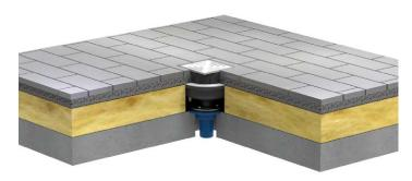
Built-in balcony drain DN 50 as basic element and slip on balcony complete drain DN 50 as extension element installed in a insulated roof. The hight-adjustable inlay grate serves as an edge to the tiled surface.
