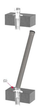
The sunken pipe inlet (1) allows the down pipe to be inserted or removed.
